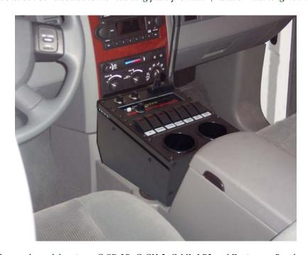
Shown with console model options: C-SP-3B, C-CH-2, C-ML-LP2 and Equipment Bracket.
